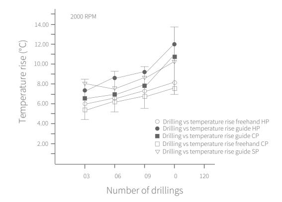
Sterilization was performed after every 3 drilling. Temperature was measured after every 30 drilling. To provide control, freehand drillings were also performed. The main question was how soon we reach the 47°C necrotic threshold, considering whether the drillings were performed freehand or guided, the roughness of the sterilization applied and drilling speed. We show only the results (means and standard deviations) for the most extreme speed here (2000 RPM), to illustrate our point:
