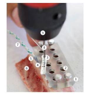
The osteotomies were performed with 2.0 mm diameter stainless steel drill bits from the SMART Kit, under 3 sterilization protocols of different roughness, at 800, 1200, 1500, and 2000 rpm (extreme speeds not occurring in real-life implant surgery were applied on purpose).
